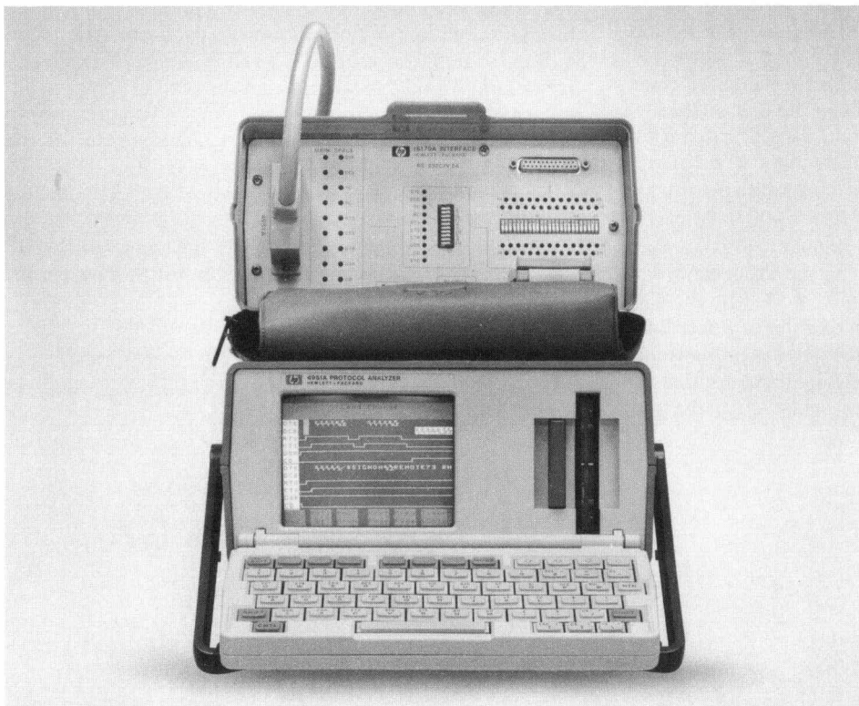
Fig. 1. The HP 4951A Protocol Analyzer is designed for field service. It has a menu-driven softkey user interface, and one softkey invokes an Autoconfigure routine that automatically determines a line's protocol, data code, speed, error checking, and other parameters.
